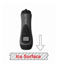
3. If there are any air pockets between the unit and ice, or the water below the ice, the unit will not work properly and will require you to try another spot, or cut a hole in the ice to use.
